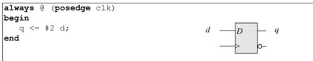
Figure A.28 Code segment using intrastatement delay with blocking assignment.
